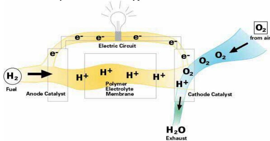
**Figure 1.2:** Basic internal operation of a fuel cell.
