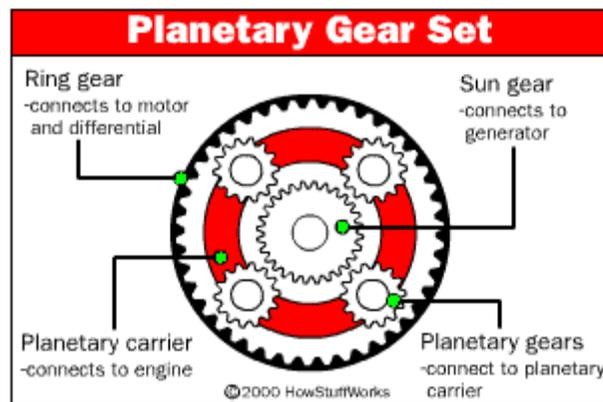
Figure 5: Planetary Gear set.
