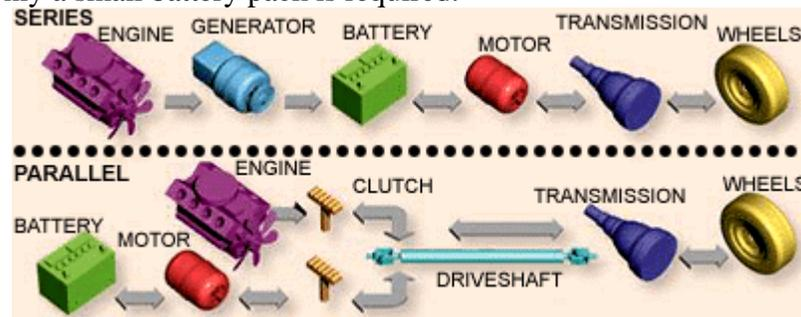
**Figure 1.1:** A model of series and parallel types.
